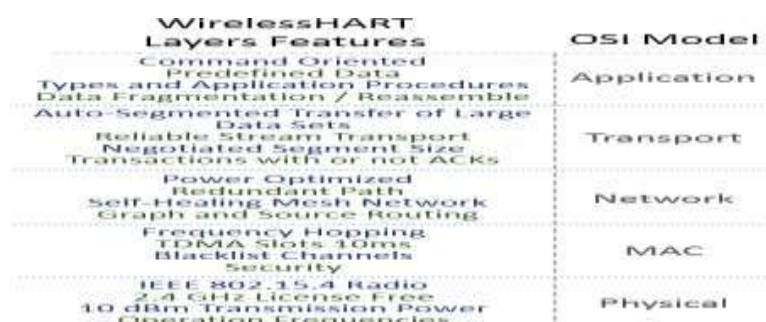
Figure. 3.12 WirelessHART Protocol Stack.
