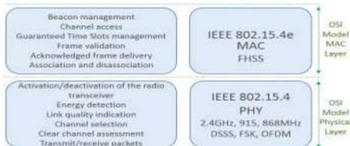
Figure 3.10 IEEE 802.15.4 compared with OSI reference model.
